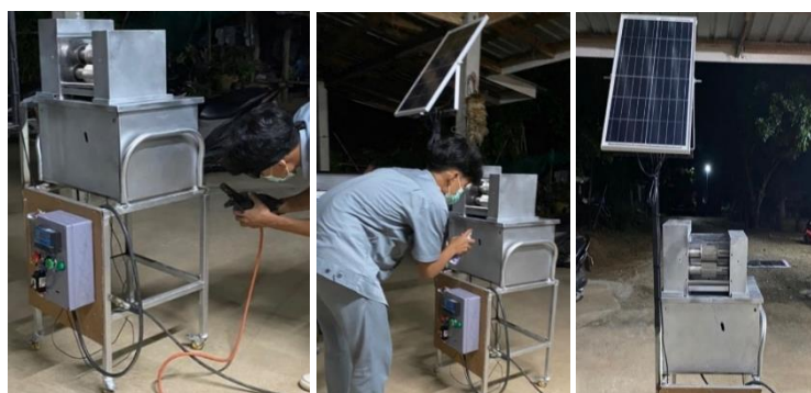
Figure 2 Building a solar sugarcane juicer
