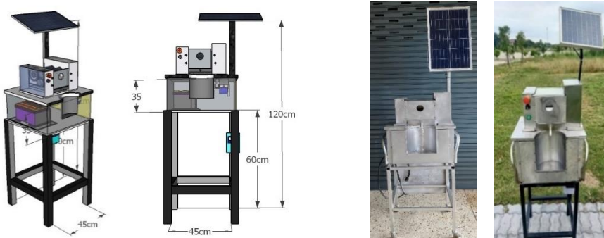
A. Structure of the sugarcane juicer
