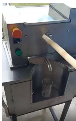
Figure 4 Testing the efficiency of a solar sugarcane juicer
